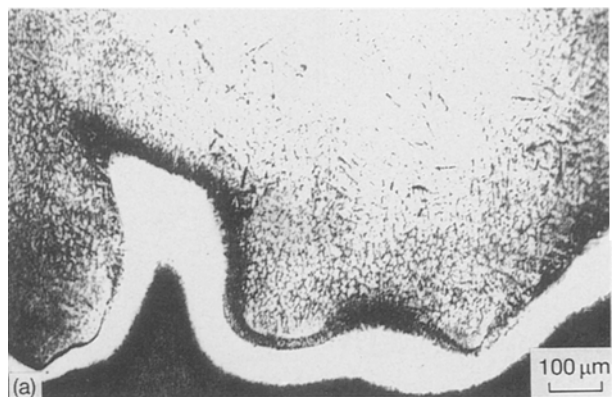
Figure 8 Laser surface molybdenum-alloyed structure of Ti-6Al-4V alloy, (a) from the melted zone, (b) showing dendritic structure.
