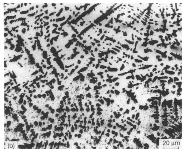
Figure 13 Laser surface niobium alloyed structure of Ti-6Al-4V alloy, (a) from the melted zone, (b) showing dendritic structure.
